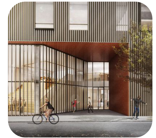
Use of directional wall and color at recessed entry
