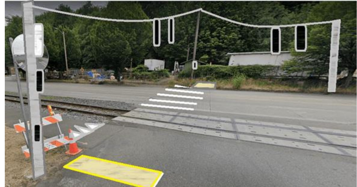
A rendering of the temporary signal at Herrings House Park driveway and West Marginal Way
