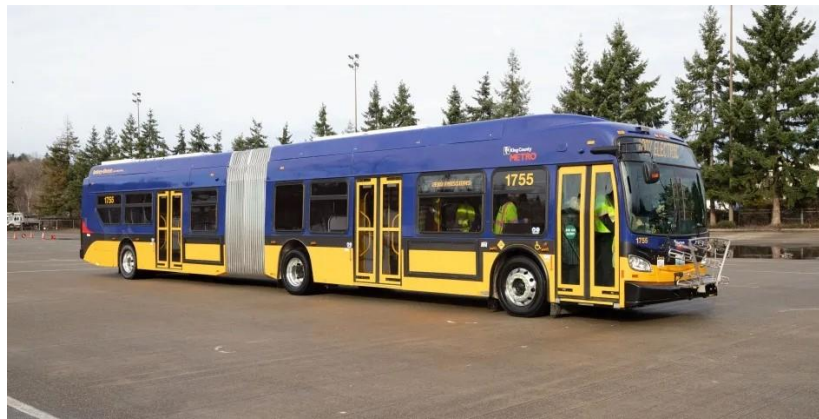
A King County Metro battery-electric bus undergoing tests. https://kingcountymetro.blog/2021/01/11/metro-invites-vendors-to-build-battery-electric-bus-charging-facility/
